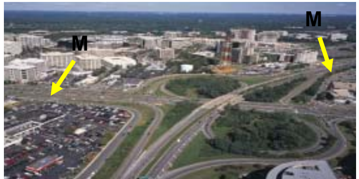
This cloverleaf at 123 and Route 7 connects two 35 MPH roads and is within the ¼ mile walking distance of two Metro Stations. By overlaying a grid system in the area traffic can be distributed and this cloverleaf can be redeveloped into a city park and 25 areas can be developed into housing and commercial space. This can become the 100% corner at Tysons.
