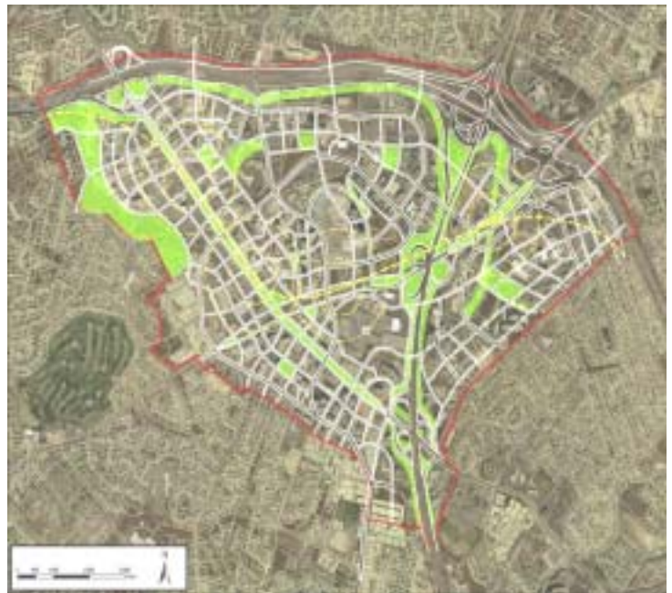
By weaving a grid into Tysons the east west traffic lanes can increase from today's 6 lanes (Rt. 7) to 30 east west lanes. Using one-way pair's traffic lights can be timed for rush-hour flow. There are currently 26 north-south lanes across Rt. 7. With a new grid there can be 84 lanes in the north-south direction. This will solve a lot of existing traffic problems. The grid can also provide up to 14,000 on street parking spaces during non-rush hour periods.
